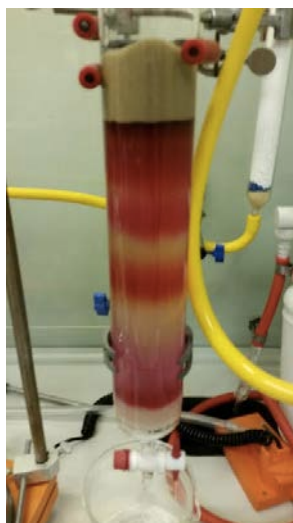
Figure 2. Column chromatography - you can see the different colour bands representing different compounds being separated.
