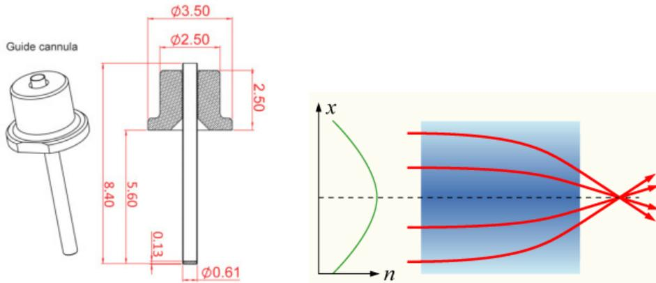
(a) Schematic and dimensions of a rod-shaped GRIN lens. (Bocarsly et al. 2015).
